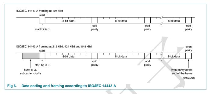
The internal CRC coprocessor calculates the CRC value based on ISO/IEC 14443 A part 3 and handles parity generation internally according to the transfer speed. Automatic parity generation can be switched off using the MfRxReg register's ParityDisable bit.
