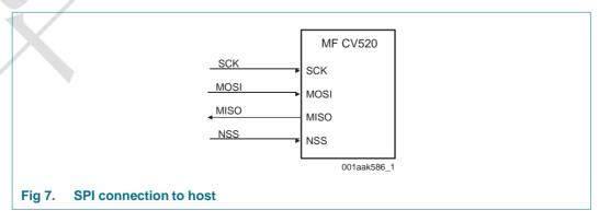
The MF CV520 acts as a slave during SPI communication. The SPI clock signal SCK must be generated by the master. Data communication from the master to the slave uses the MOSI line. The MISO line is used to send data from the MF CV520 to the master.
